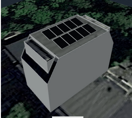
3D model of solar arrangement now 2x6panels
